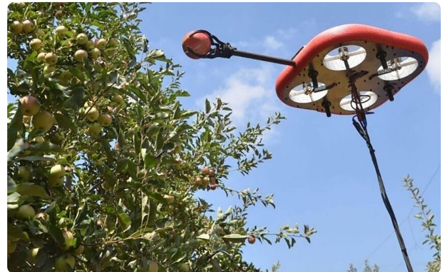
Flying Fruit Pickers: Intelligent fruit picking drones analyze ripeness, color, and size before initiating gentle tactile harvest grips (Tevel).
